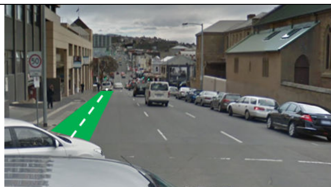
Between Macquarie St and Melville St the roadway would need to be reduced from 3 narrow to 2 wider travel lanes, a similar treatment as Mollie St.
