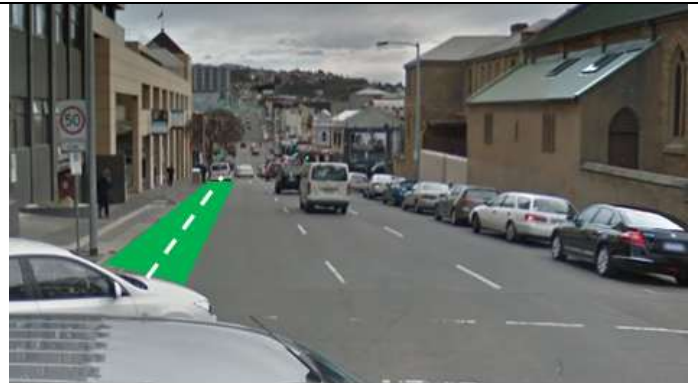
Between Macquarie St and Melville St the roadway would need to be reduced from 3 narrow to 2 wider travel lanes, a similar treatment as Molle St.
